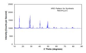
Fig. 2. XRD pattern of Nd(OH)<sub>3</sub>(micro cr) used in solubility experiments in this study.
