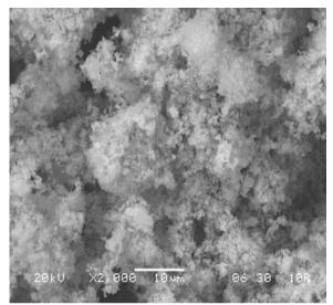
Fig. 1A. SEM image of the starting material used in experiments in this study.
