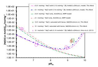
Fig. 3. A plot showing Nd(III)/Am(III) concentrations as a function of pHm in low ionic strength range.
